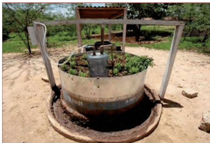
Figure 25.1 Sertanejo biodigestor built in the Brazilian semi-arid region. Source: Mattos & Farias (2011)
